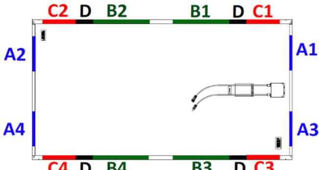
**Table 1:** Approved module clamping/direct fixation zones
