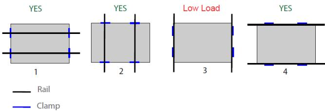
Configurations 1 and 2 show mounting with rail support, 3 and 4 show mounting without rail support. In "With Rail Support" the rails becomes conventional or rails transverse while "Without Rail Support" becomes end mounted in long or short side. In the case when the glass deflects it would not deflect in the rails for additional support.
